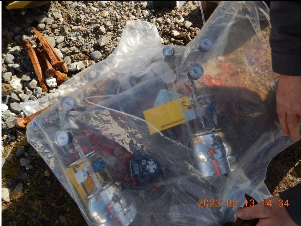
5 SSI -1 @ 5' depth - soil vapor sampling 1-Liter canisters (duplicate sample being collected)
