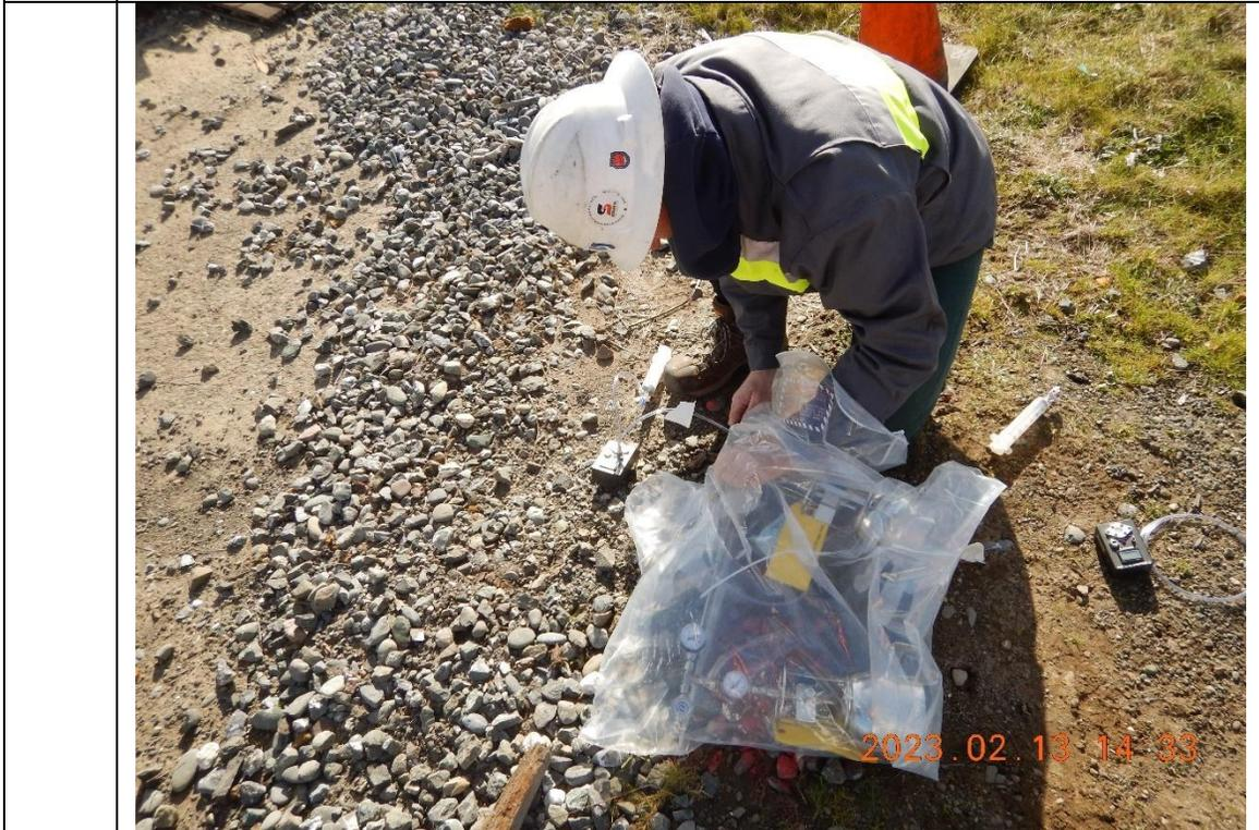
4 Soil vapor sampling at SSI-1 @ 5' depth
