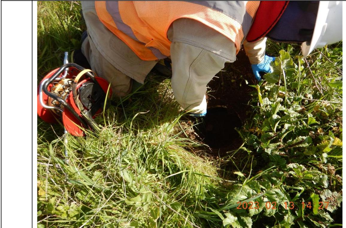
8 Kennedy/Jenks' Mike McLeod checks water level at well W-3.16R – well depth 24.5' – level 4.53' below Top of casing
