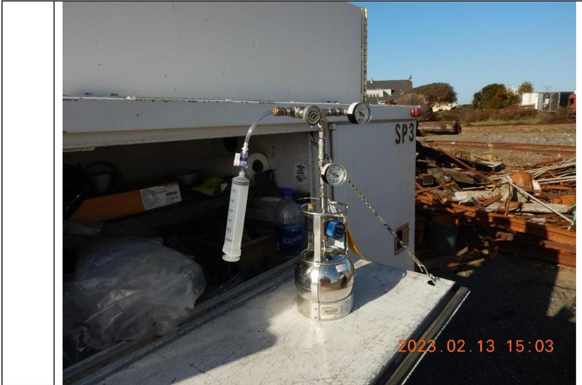
7 TEG Chris Van Senus performs a vacuum leak check on the sample train for SSI-2
